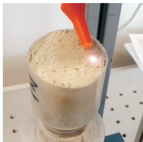
A typical measurement at a concrete core. The volume around the plasma is purged with Helium.
